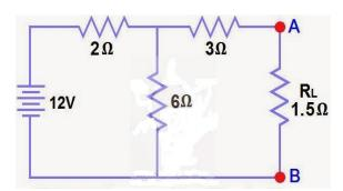
21. Find the value of  $R_{\rm L}$  for maximum power in the circuit of fig given below. Also find the maximum power.
