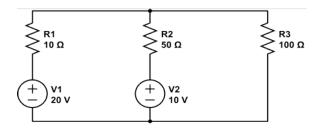
18. Calculate the total current I<sub>3</sub> using nodal analysis
