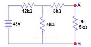
20. Calculate the load current and load voltage using Norton's equivalent circuit.
